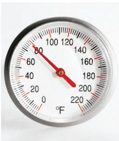
The first place to start is: Cure Temperature. While some epoxies will cure at room temperature, many will require an elevated temperature to initiate the chemical curing reaction. Suggested *minimum* temperatures and times are listed under the “minimum cure” section of the datasheet.
